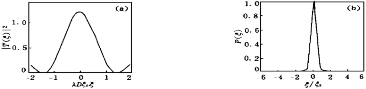
Fig. 1 (a) Squared modulus of spatial-frequency spectrum of pupil function with U < 4 , (b) Normalized optical transfer function with U < 4
