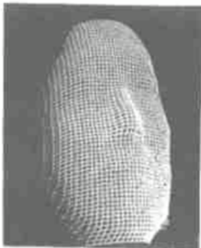
Fig. 6 Mesh plot of 3D image of a human face approximated by B-spline
