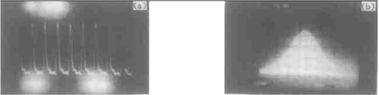
Fig. 6 Mode-locking pulses. (a) The part of the mode-locking pulses train, (b) The whole envelope of the mode-pulses
