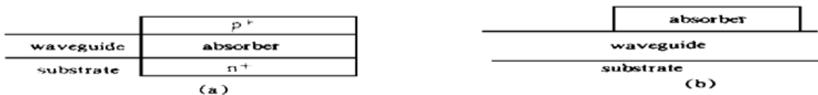
Fig. 1 Side view of couple structure of waveguide and photodetector. (a) Butt-coupled, (b) Vertical-coupled absorber
