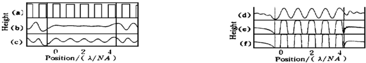
Fig. 1 The supposed sample surface as computation mode (a) and some computation results (b~ f). (a) the supposed sample surface parameters: height= \lambda/10 , sample's period varies from 0.5 \times \lambda/NA to 10 \times \lambda/NA (b) computation result of sample surface while sample's period equals 0.5 \times \lambda/NA . The measured surface height is approximately 0. (c) period= 0.6 \times \lambda/NA , measured height= 24.9% of the ideal sample height. (d) period= 1.0 \times \lambda/NA , measured height= 69.9%. (e) period= 4.0 \times \lambda/NA , measured height= 94.2%. (f) period= 10.0 \times \lambda/NA , measured height= 97.7%
