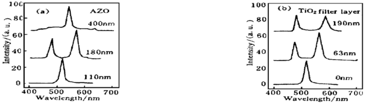
Fig. 5 EL spectra of microcavity with different thickness of AZO (a) and TiO 2 filler layer (b)
