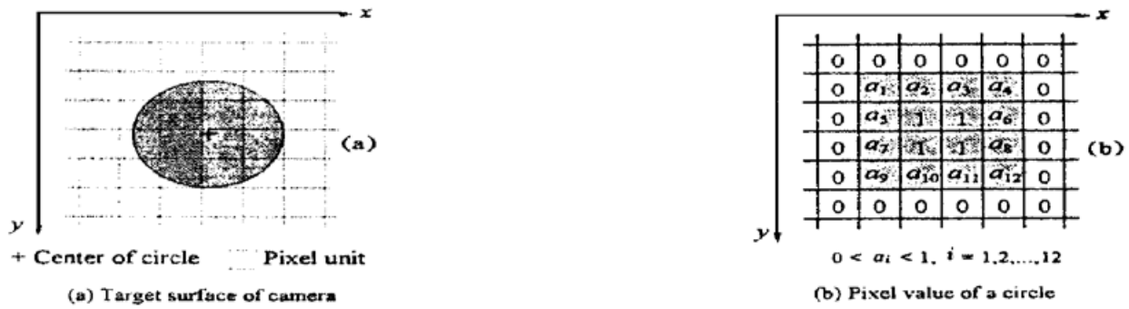
Fig. 1 The image of a circle captured by camera. (a) Target surface of camera, (b) Pixel value of a circle
