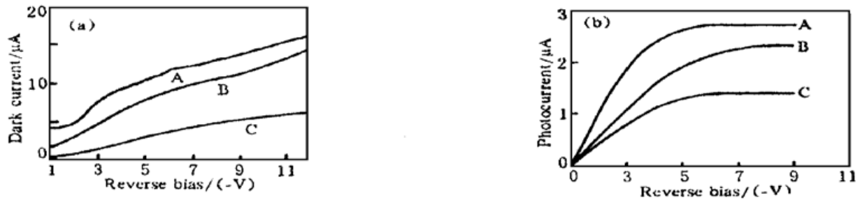
Fig. 3 Test result of dark current and photocurrent of photodetector. The length of absorbed area: A: 4 mm, B: 3 mm, C: 1 mm, width: 20 \mu\text{m} . (a) Relation of dark current with reverse bias and area, (b) Relation of photocurrent with reverse bias and area
