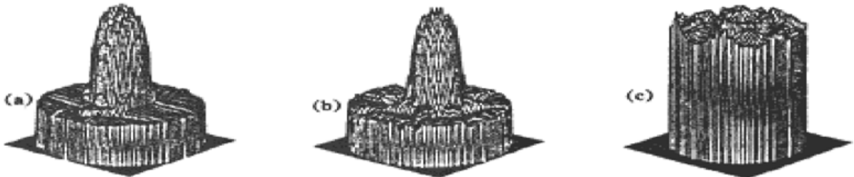
Fig. 4 Original intensity distribution of different plane of Model I. (a) Z = 0 plane, (b) Z = 5 plane, (c) Z = 10 plane
