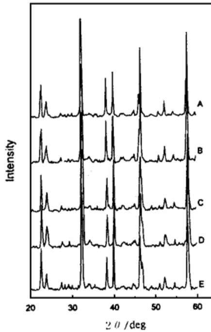
Fig. 1 XRD patterns of Nd 0.9 Ca 0.1 Ba 2 Cu 3 O 6+x samples
