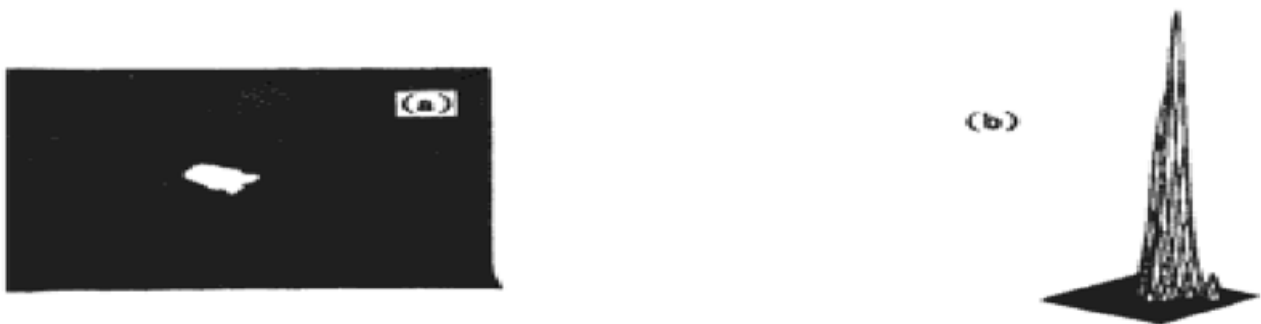
Fig. 4 (a) Correlation output and (b) its corresponding 3-D plot obtained using wavelet matched filter
