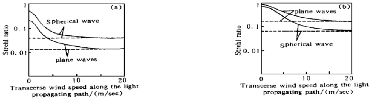
Fig. 4 Relationship between Strehl ratio of the 37-element adaptive optics system and transverse wind speed along the light propagation path. The dashed lines are corresponding to open-loop condition. (a): C_n^2 is 1.28 \times 10^{-13} \text{ m}^{-2/3} , (b) C_n^2 = 2.77 \times 10^{-14} \text{ m}^{-2/3}
