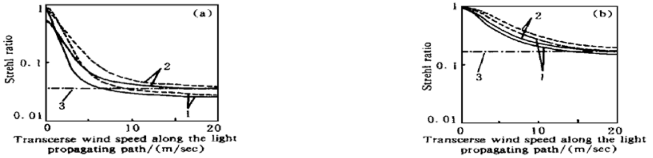
Fig. 3 Relationship between Strehl ratio SR and transverse wind speed along the light propagation path. Lines 1, 2, 3 are corresponding to ideal adaptive optics system, adaptive optics system with finite bandwidth, and open-loop conditions. The solid lines are corresponding to spherical wave while the dashed lines to plane wave. (a): r_0 is 0.02 m, (b): r_0 is 0.05 m
