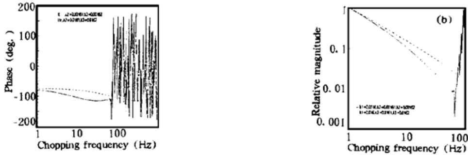
Fig. 5 Theoretical calculation of photoacoustic phase (a) and magnitude (b) versus chopping frequency f for different thermal diffusivity coefficient for each layer
