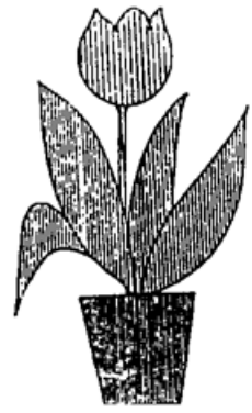
Fig. 1 Red tulip with green leaves growing in a blue pot. The color are encoded in three gratings with about 80, 95 and 100 lines/mm. Example given by R. W. Wood in Nature 1899
