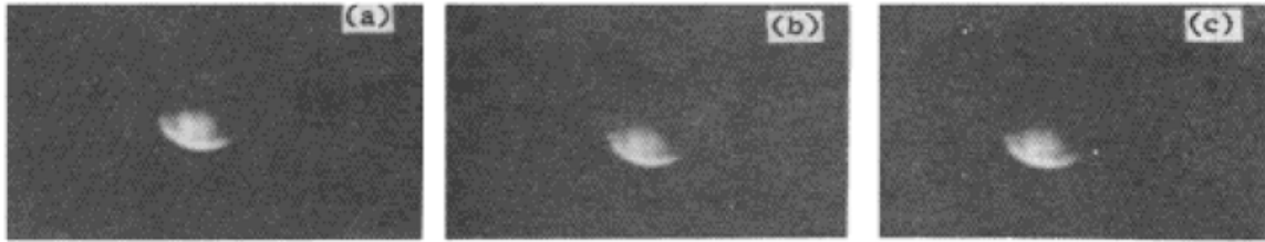
Fig. 5 The photograph of SPPC light beam observed on the screen S at t = 60 ms (a); 100 ms (b); and 140 ms (c)
