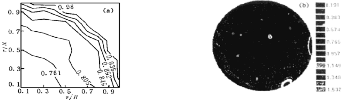
Fig. 5 The distribution of the deposited energy density and pumping induced thermal aberration, r/R is normalized radius.
