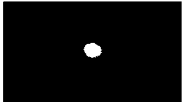
Fig. 5 Laser beam spot recorded by CCD
