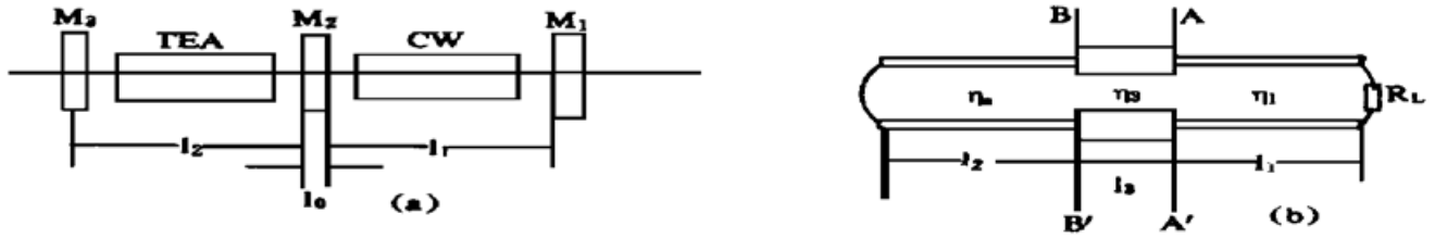
Fig. 1 (a) Schematic of composite cavity injection locking laser, (b) Its equivalent circuit
