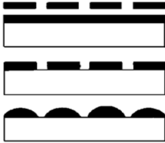
Fig. 1 Fabrication sequence of the refractive microlens Fig. 2 Schematic representation of design model
