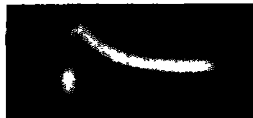
Fig. 7 Biasing temperature = 52^\circ\text{C} He-Ne laser and TEA \text{CO}_2 laser simultaneously incident upon \text{VO}_2 film
