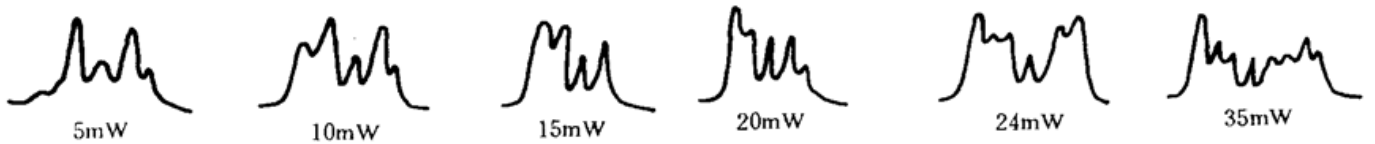
Fig. 10 Evolution of dark spatial solitons with different laser intensity. With increase of laser intensity, the pairs of dark spatial solitons increase
