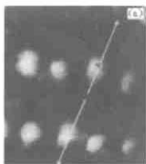
Fig. 6 STM images of the recorded film on a pregrooved polycarbonate substrate before and after laser irradiation; (a) STM images; (b) A line scan across the bubble
