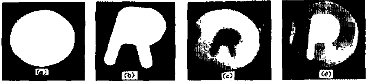
Fig. 5 (a) self-pumped phase conjugate image of the uniform Gaussian beam impressed on the pumping beam, (b) complete phase conjugate image of "R" impressed on the signal beam, (c) image subtraction, (d) image addition
