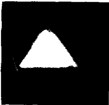
Fig. 6 Experimental result for the edge-enhancement output in the signal beam. A "triangle" and a "uniform Gaussian beam" are impressed on the pumping and signal beams, respectively
