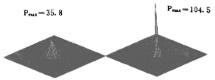
Fig. 3 Beam intensity distribution before and after compensation, pmax is relative peak value
