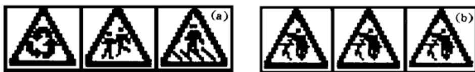
Fig. 3 The performance of Hopfield model when 3 traffic signs being as stored patterns. (a) 3 stored patterns (b) recalled patterns
