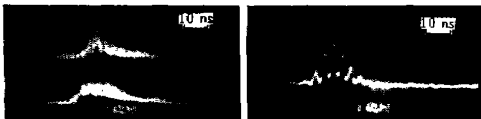
Fig. 3 Oscilloscope traces of injection mode-locking (green laser line). (a) Real-time trace of the temporal waveforms of the injection locked slave laser (bottom) and the injected seed laser (top). (b) Single-shot trace of the temporal waveform of the injection mode-locked pulses.
