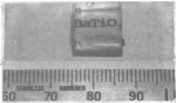
Fig. 4 Polished cube after mechanical and electropolishing
