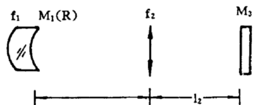
Fig. 2 Optical schematic layout of the pump resonator
