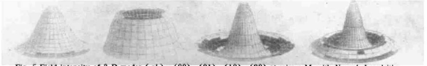
Fig. 5 Field intensity of 3-D modes (pl) = (00), (01), (10), (20) at mirror M_1 with N_f = 4.1 and its confocal resonator N = 0.56
