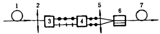
Fig. 5 Scheme of a novel polarization-insensitive TW-SOA
