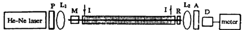
Fig. 5 Experimental setup for the measurement of Verdet constant. p: polarizer, L_1, L_2 : \times 10 microscope objective, M: positioner, R: rotative disk, A: analyzer, D: Si-Pin detector, Meter: optical power indicator
