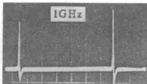
Fig. 5 Optical spectrum of single-mode operation at 1,064 \mu\text{m} measured by using a scanning confocal interferometer with 25 MHz resolution and a 1 GHz free spectral range
