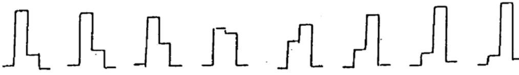
Fig. 7 Output signal of an element at eight different stages of scanning
