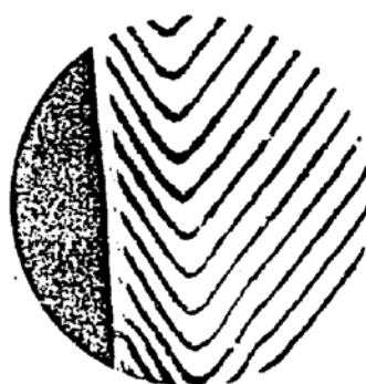
Fig. 4 Interferogram of heating plate by experimental setup in Fig. 2
