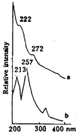
Fig. 2 Absorption spectra of (a) Sample A coated on fused silica, (b) C_{60} in hexane solution [2]
