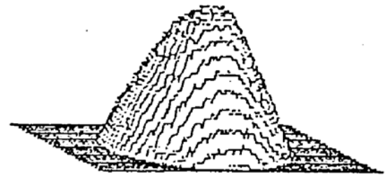
Fig. 3 CW output of \text{TEM}_{00} -mode Nd:BGO laser
