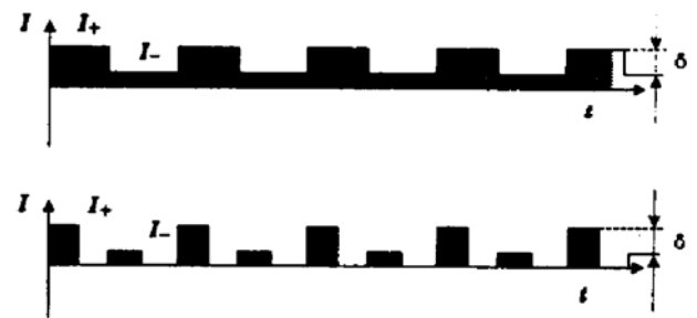
Fig. 4 Square waves obtained by photodetector
