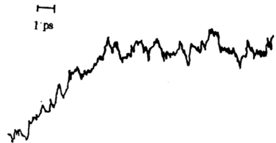
Fig. 3 E-O sampling when distance between exciting and sampling beam is 1.0 mm, the 10~90% risetime is about 5 ps
