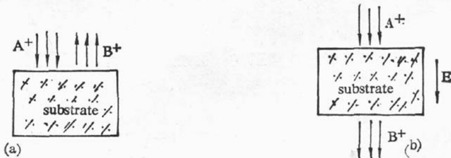
Fig. 2 The form of ion escaping from substrate (a) diffusion; (b) electromigration
