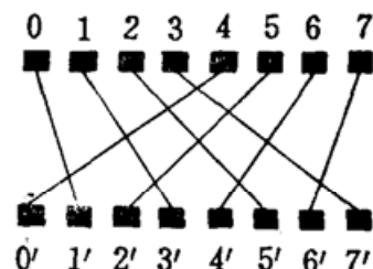
Fig. 4 Right perfect shuffle interconnection network
