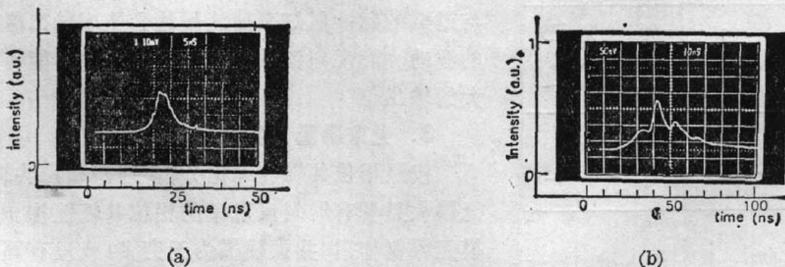
Fig. 4 Photocurrent oscillograms for lasing pulse obtained by resonator with (a) l_1=440 \text{ mm} , L_1=600 \text{ mm} ; (b) l_2=1450 \text{ mm} , L_2=1850 \text{ mm}
