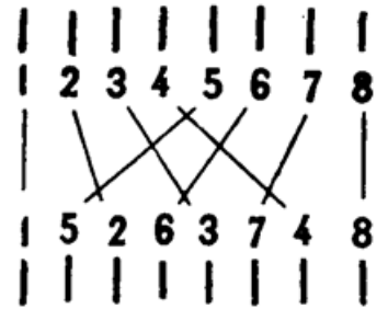
Fig. 1 Perfect shuffle permutation of eight inputs
