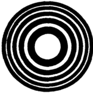
Fig. 2 Fresnel zone plate
