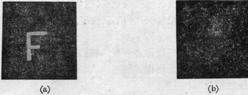
Fig. 3 The experiment by character letter F with a diffuser (a) Letter F; (b) The output from FHF by the object wave after passing through a moving diffuser
