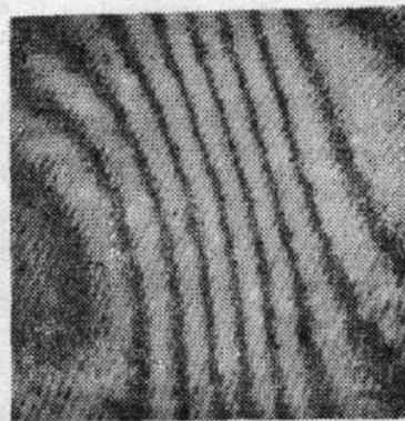
Fig. 4 Interferogram of a spheric reflective sample
