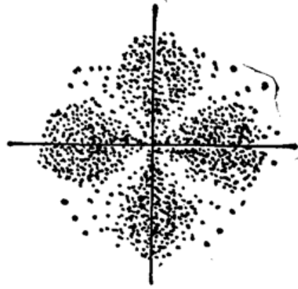
Fig. 2 Small-angle light scattering pattern of unusual spherulite
