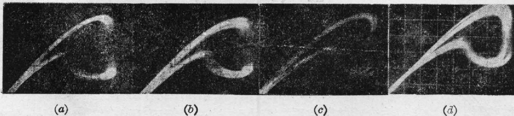
Fig. 3 Oscilloscope traces of bistable operation of ZnSe
