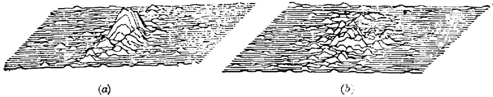
Fig. 8 The energy profile at image plane with perturbation, open-looped, amplitude (a) \pm 1\lambda ; (b) \pm 2\lambda
