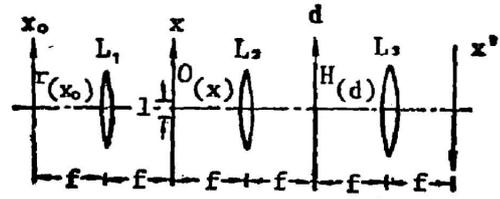
Fig. 1 One-dimension partially coherent processing system
