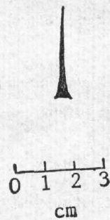
Fig. 3 Near-field plexiglass burn pattern (output power 7 kW)
