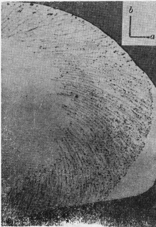
Fig. 6 Inclusion distribution in c -axis crystal (0 0 1) wafer 90 \times
